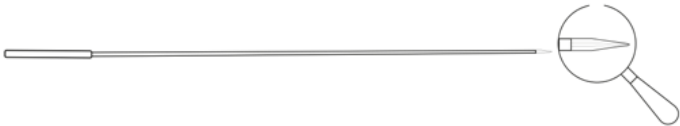
Figure 12: Scheme of a Packed Integrated Emitter Capillary.
