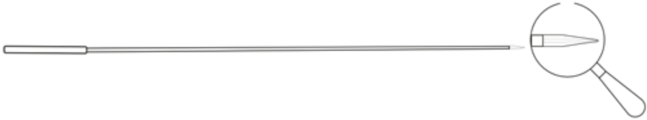
Figure 11: Scheme of an Empty Integrated Emitter Capillary.
