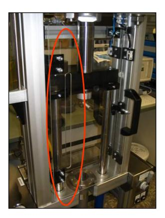
The front door of the new instrument features an integrated capillary guidance. It allows to control the inlet capillary and its endfitting from the outside of the closed / secured packing cabinet and protects them from getting damaged by the moving parts.
