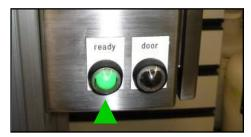
*Green Indicator* shows when the system is pressurized and ready for column packing.
