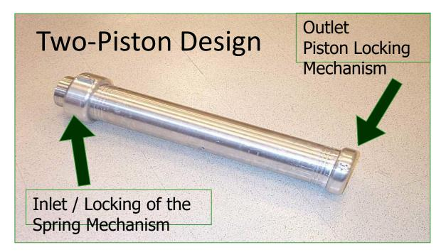
Same piston design as for the 25 and 50mm I.D. Spring columns
