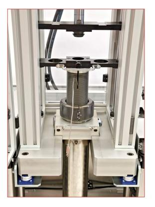
A hinged column bracket with handles is used to place the 4" Spring<sup>®</sup> Column inside the Multipacker<sup>®</sup>, allowing an easy handling and transportation of the column.
