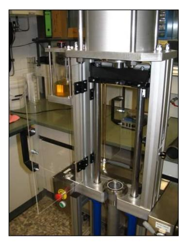
The new Multipacker features individual safety doors for protection at the front and back side of the instrument (opening 90° to the same side). This allows full and easy access to the column hardware for preparation and handling.
