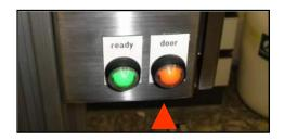
Orange Indicator shows when the packing adapter has stopped and has been secured so that the safety door can be opened without danger.
