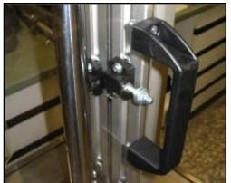
Pneumatic Door Sensor to automatically depressurize the system when the door is opened.
