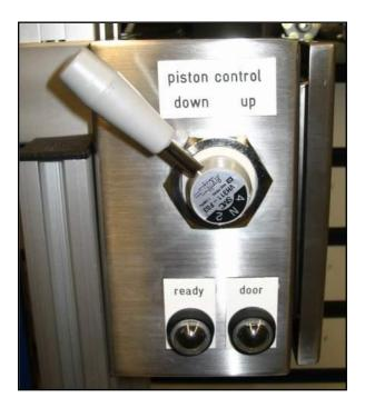
Heavy duty switching valve allows easy and reliable control of the pneumatic piston's movement.
