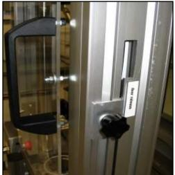
Security Glass Safety Doors with Magnetic Interlock (antistatic and solvent resistent).
