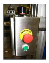
Door Release Sensor that (when aligned with packing adapter) allows the door to be opened without the system depressurizing (necessary for locking the pressurized packed column).
